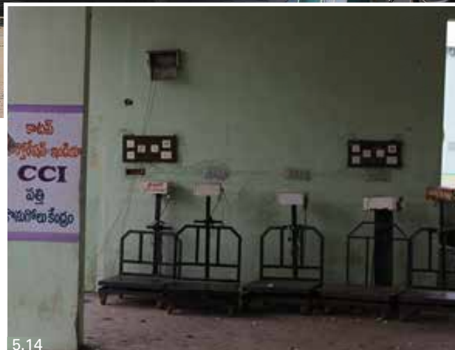
Photos 5.12- to 5.14: Weighting scale technologies – electronic weighing bridge, electronic weighing platform and traditional manual weighing balance. Fair weight measurement, an important parameter of terms of trade, is compromised by the use of manual scales and manipulation by traders.
